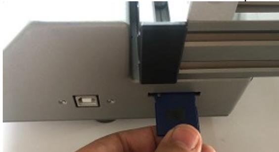
3.3. Turn on the printer. The printer would start flashing automatically. After finishing flashing, printer would come back to starting screen as below. Please delete firmware inside SD card.
